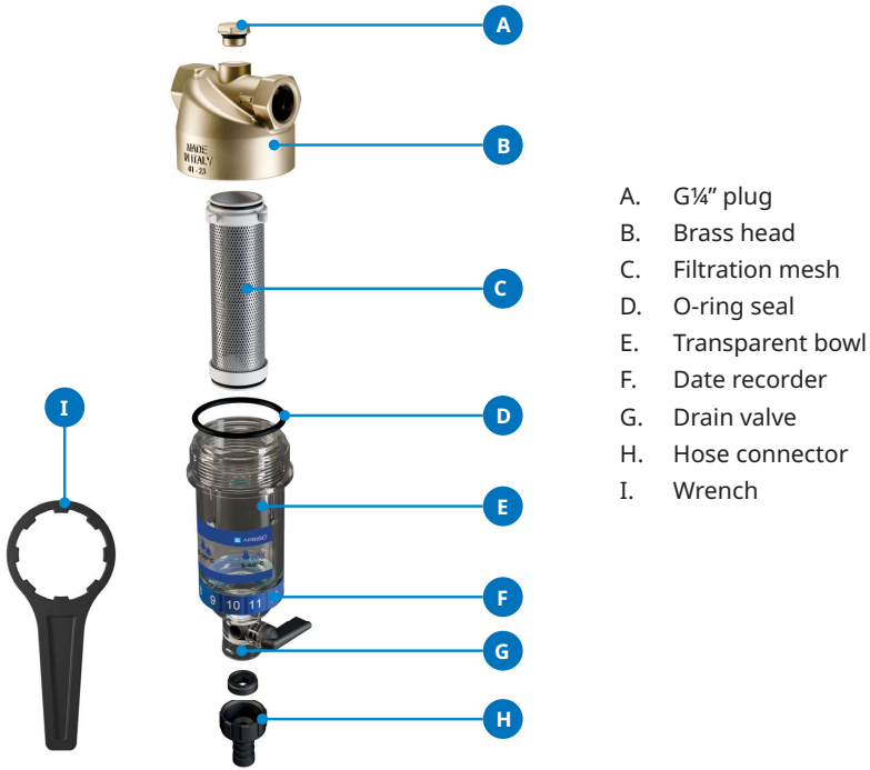
Fig. 2. Construction of the AWF water filter
