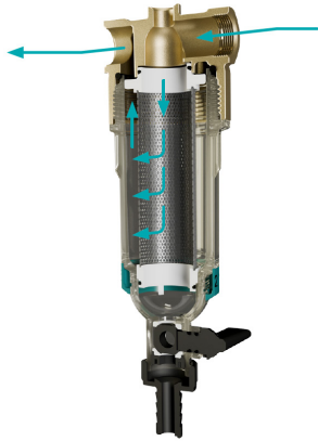
Fig. 1. Diagram of water flow through the AWF filter
