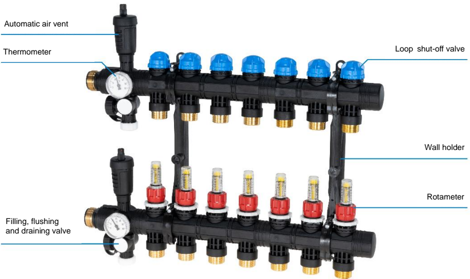
Figure 2: Construction of the ProCalida EF1 manifold
